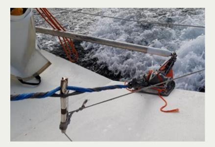
We put on both runners, then steered the boat up head to wind to slow it down. The plan was to lever the rudder back into place and tie it forwards into the cup somehow.
